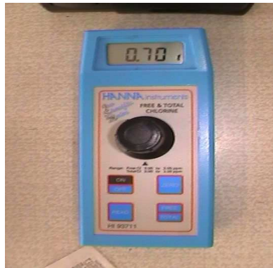
Figure 1.1 Instruments used to find the free & total chlorine values
