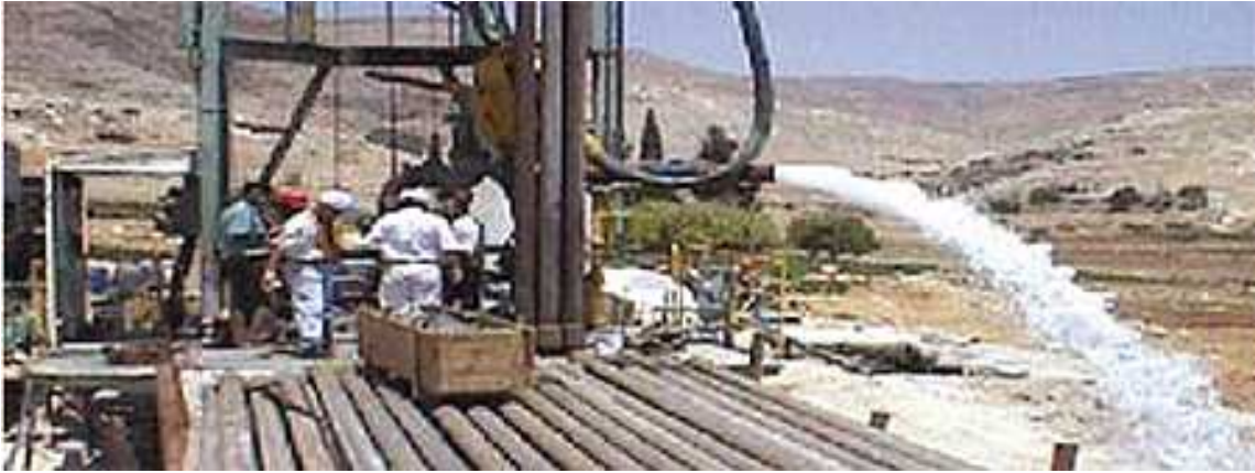
Figure 4.2: Well No. 6-Final Test at 330 m 3 /h Discharge Rate (19-21 July, 1999)
